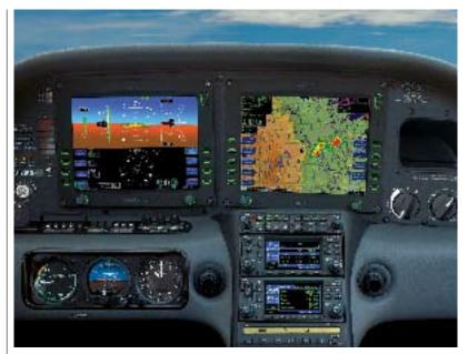
The first use of EFIS for civil aviation was in the Boeing 757 and 767 in 1978. Boeing began development of the 757 and certification of the electronic cockpit. In general aviation, the Beechcraft Starship was the early adopter for electronics instrumentation, with 27 CRT displays that mimicked the electromechanical instrumentation, which was introduced in 1988.
