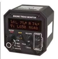
screen. With a four- or six-cylinder engine, the instrument graphically presents the data for each jug using four or six vertical bars. Many monitors also can display an additional bar dedicated to another engine parameter, like oil temperature or turbine inlet temperature (TIT) for a turbocharged aircraft.
